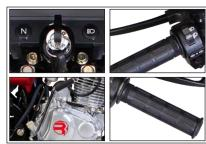
**Riding Operation** - After starting and preheating, return main and side stand. Now hold clutch lever and pull it towards yourself. Then press pedal gear change with left foot and shift to the first gear.
